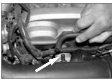
5. Disconnect the crank case vent hose from the stock intake tube as shown.
