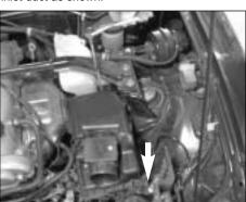
8. Loosen and remove the hex bolt and nut tha secure the air cleaner assembly as shown.
