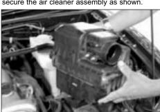
9. Pull upwards to remove the air cleaner assembly as shown.
