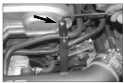
17. Using the provided hex bolt secure the bracket to the cam cover as shown.
