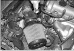
19. Install the K&N Filtercharger onto the mass air sensor, then, tighten the hose clamp as shown.
