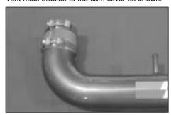
12. Install the silicone step hose and hose clamps onto the K&N intake tube as shown.
