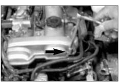
11. Remove the bolt that secures the crank case vent hose bracket to the cam cover as shown.
