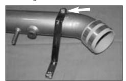
15. Install the "Z" bracket onto the K&N intake tube using the provided hardware as shown.
